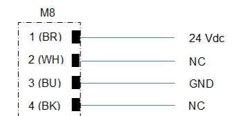
Figure 2 - Detailed wiring instructions
